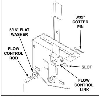
Hook free end of flow control rod through hole in slide gate bracket located near bottom of hopper. See figure 9.
